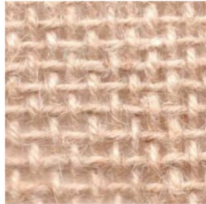
Fig. 1. Ramie woven with S12/3 type yarn
